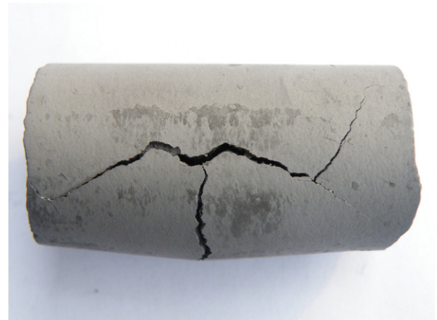
Fig. 14. Thermal debinding defects of \Phi 36 mm rod.
