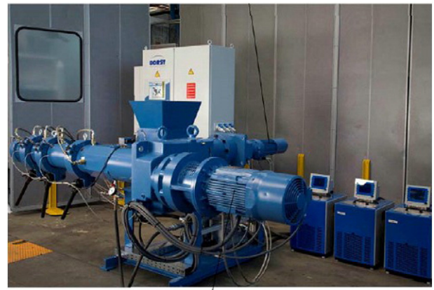
Fig. 2. A photograph showing the extrusion molding equipment.
