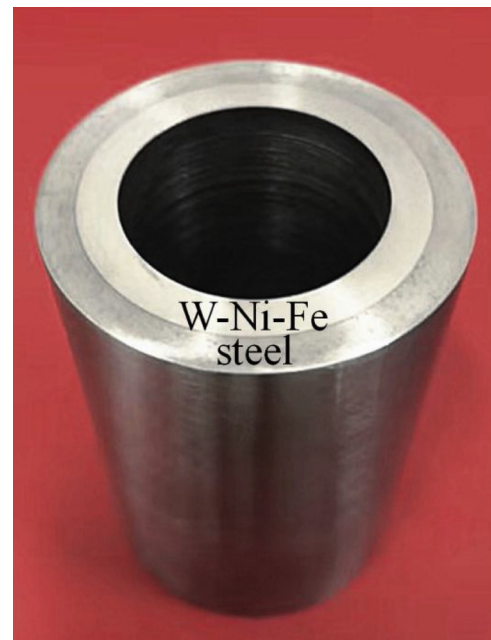
Fig. 2. HIP bonded W–Ni–Fe/steel joint mock-up after removing canning materials.
